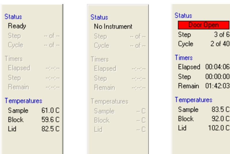
Figure 7-1 The run-status box indicates whether the instrument is ready.
